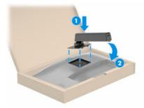
4. Attach the base to the stand (1) and tighten the screw (2).
