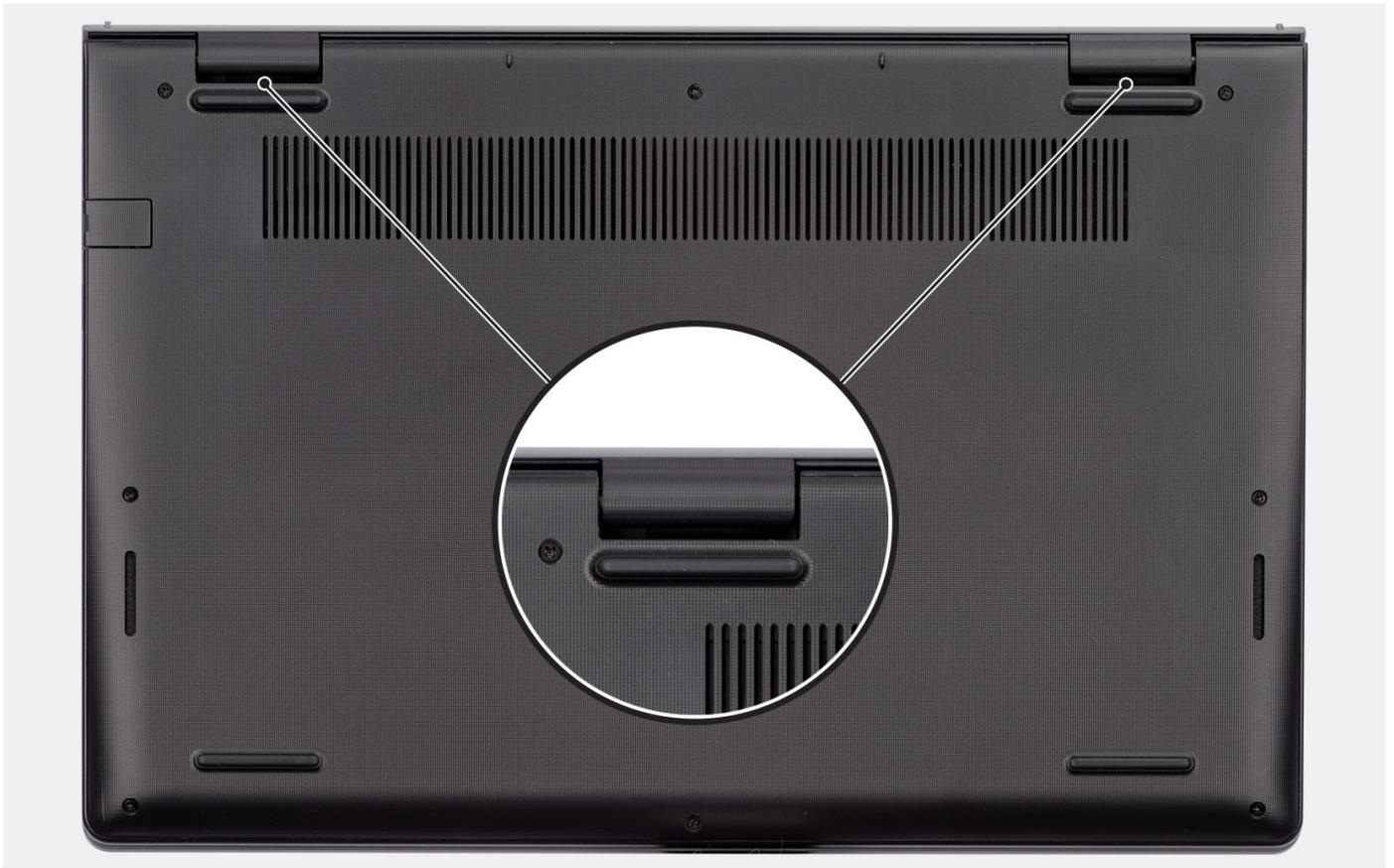
3. Pry open the top side of the base cover and continue working on the left and right sides to open the base cover.
