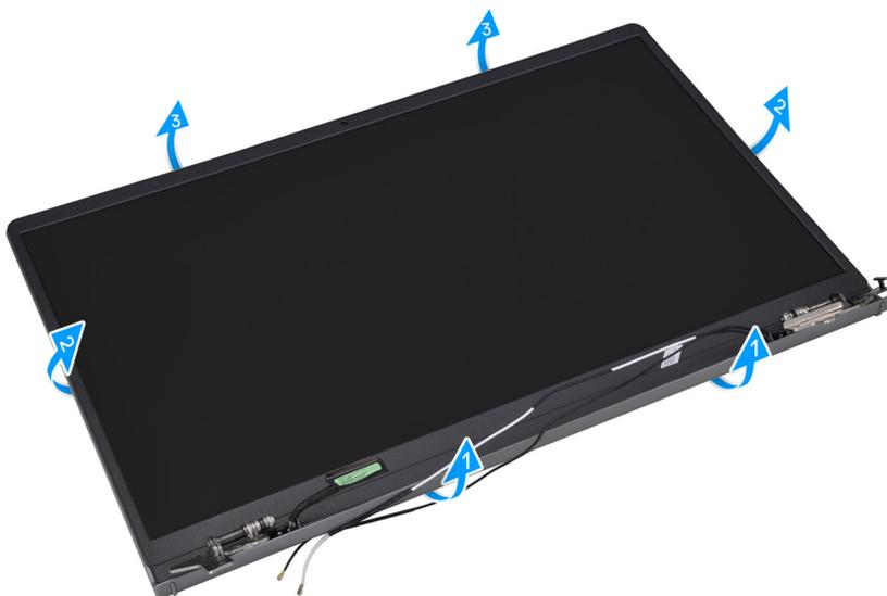
4. Lift and remove the display bezel from the display assembly.
