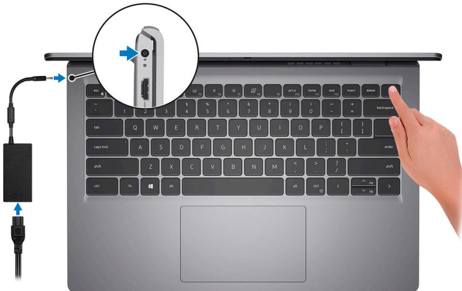
**NOTE:** To conserve battery power, the battery might enter power saving mode. Connect the power adapter and press the power button to turn on the computer.
