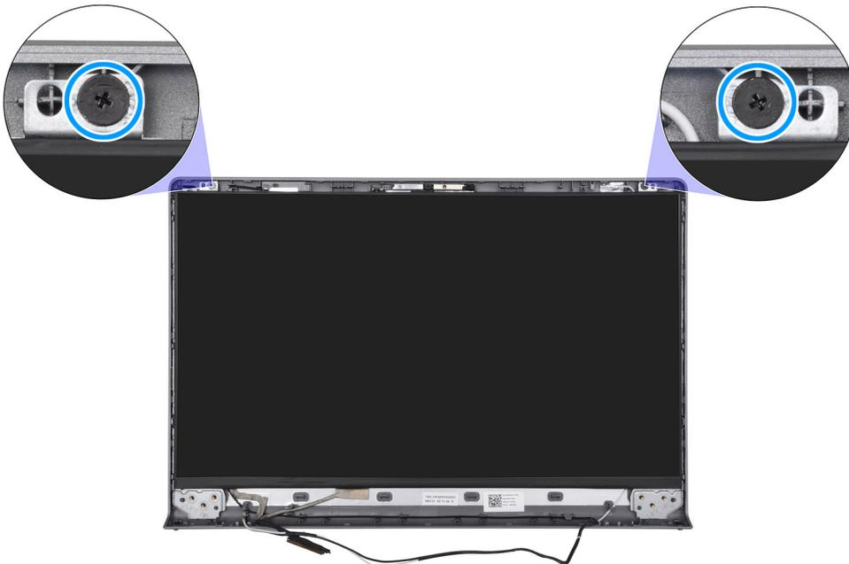
2. Using a plastic scribe, pry the display panel from the bottom-right corner.
