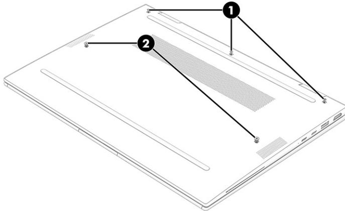
2. Use a nonmarking, nonconductive tool to release the edges of the bottom cover from the computer (1).
