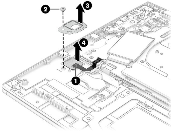
Reverse this procedure to install the fingerprint reader board.
