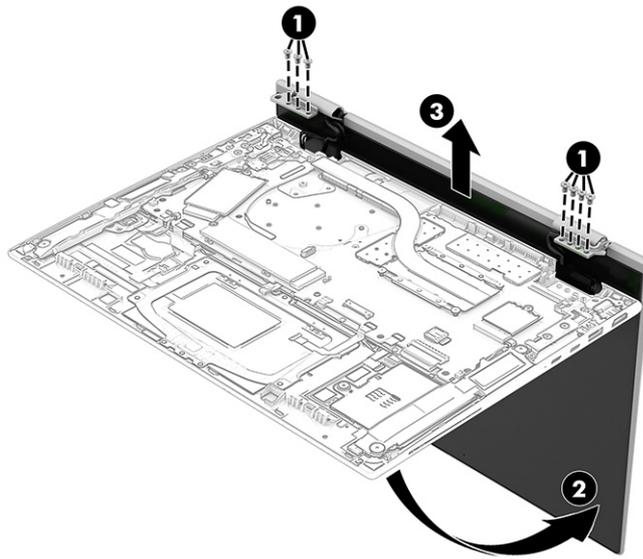
Reverse this procedure to reassemble and replace the display assembly.
