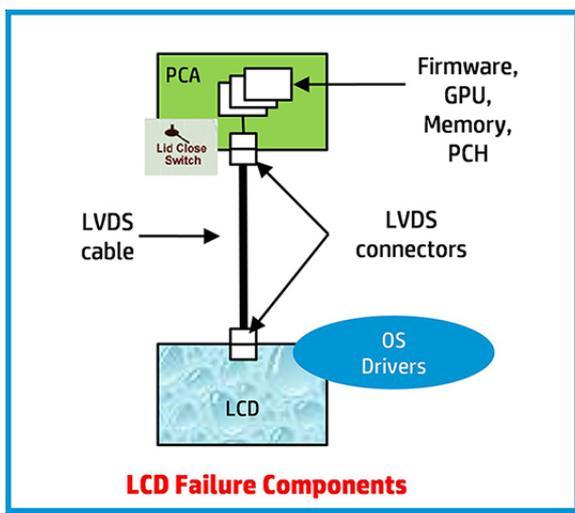
**NOTE:** The lid close switch is a Hall-effect sensor located in the top cover. When the display is closed, the sensor acts like a switch is closed. A notebook can force a video output to an external monitor, or go to
