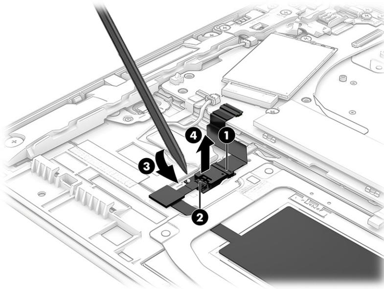
Reverse this procedure to install the NFC module.
