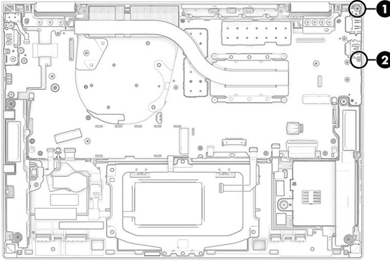
4. Remove the SIM card insert from the computer (1).
