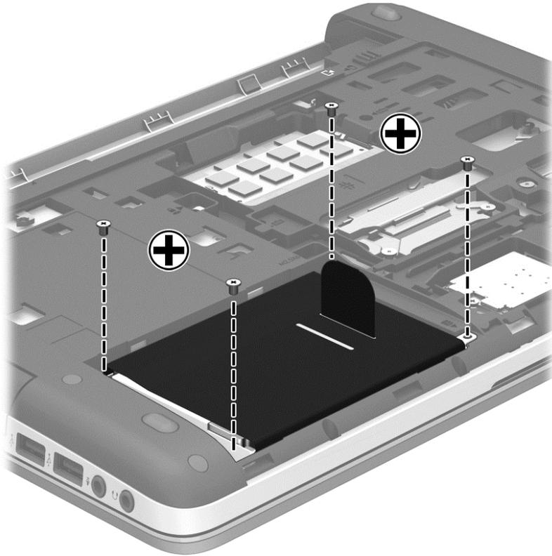
7. Pull the hard drive tab (1) towards the side of the computer to disconnect the hard drive.
