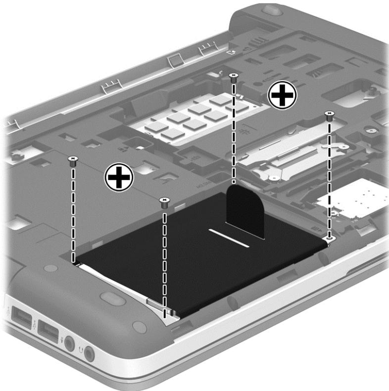
4. Replace the service cover (see [Removing or replacing the service cover on page 38](#)).
