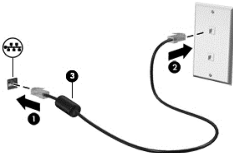
**⚠ WARNING!** To reduce the risk of electric shock, fire, or damage to the equipment, do not plug a modem or telephone cable into the RJ-45 (network) jack.
