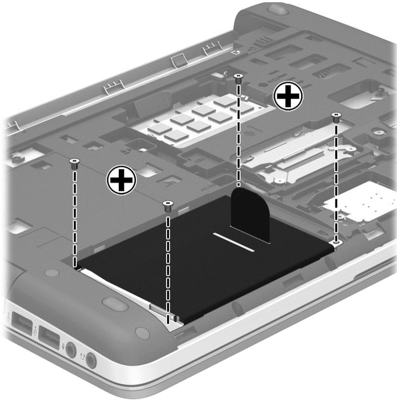
9. Pull the hard drive tab (1) towards the side of the computer to disconnect the hard drive.
