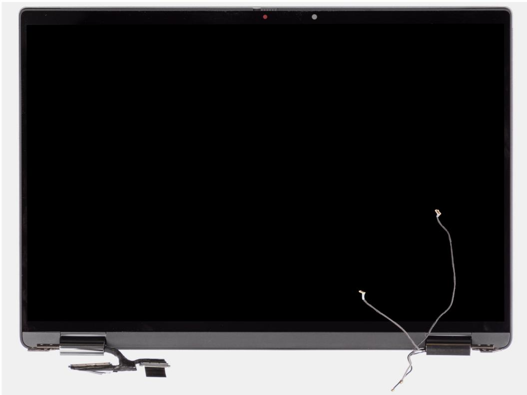
**Figure 51. Display assembly with WWAN-antenna cables**
