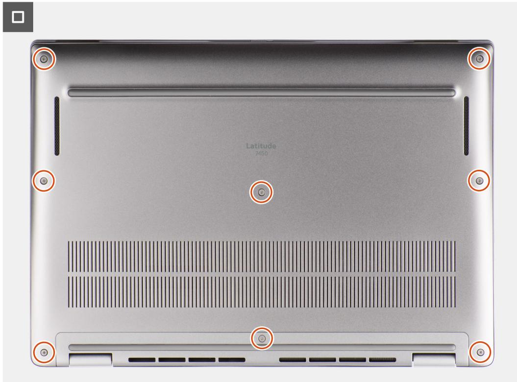
**Figure 21. Installing the base cover**
