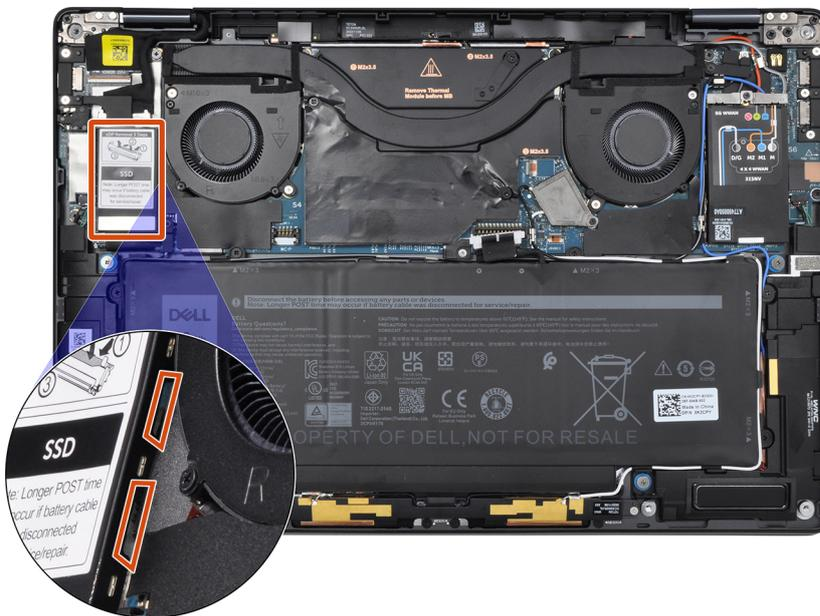
2. Remove the single (M1.2x1.5) screw that secures the solid-state drive to the system board.
