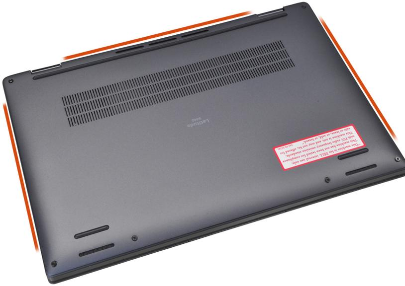
4. Hold the left and right sides of the base cover, and remove the base cover from the system.
