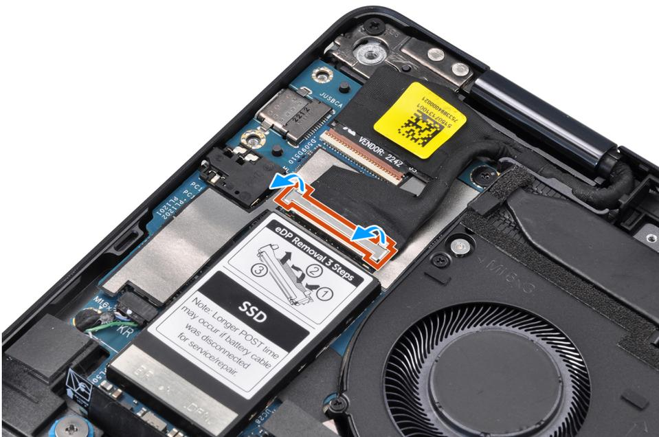
7. For systems shipped with WWAN, unroute the WWAN antenna cables from their routing guides on the system board.
