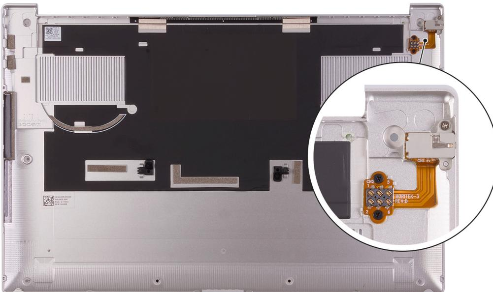
**NOTE:** Ensure to remove the protective rubber cover from audio jack pin before replacing the base cover.
