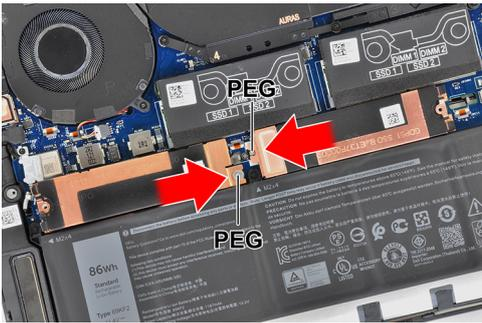
4. Align the screw hole on the solid-state drive thermal bracket with the peg on the system board.
