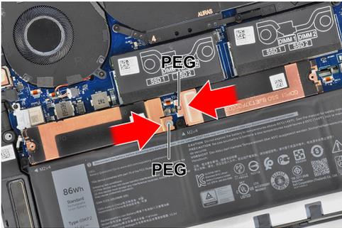
3. Slide and remove the solid-state drive 1 from the solid-state drive slot.
