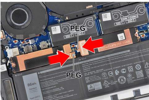
3. Slide and remove the solid-state drive 2 from the solid-state drive slot.
