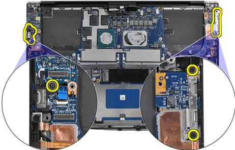
12. Open the latch, and disconnect the keyboard-control board cable from the system board.
