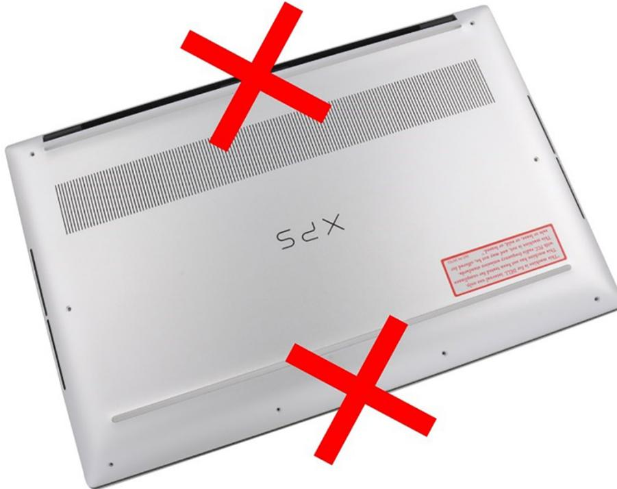
3. Grasp the left side and the right side of the base cover and remove the base cover from the palm-rest and keyboard assembly.
