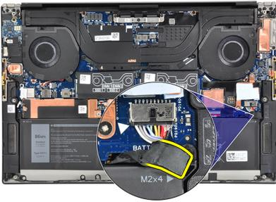
The following image indicates the location of the battery and provides a visual representation of the removal procedure.
