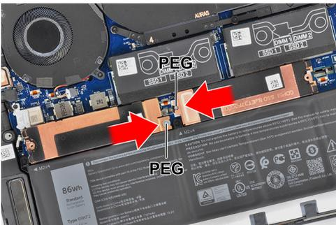
4. Replace the screw (M2x2) that secures the solid-state drive thermal bracket and the solid-state drive 2 to the system board.
