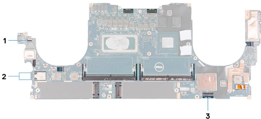
**Figure 1. System-board connectors**
