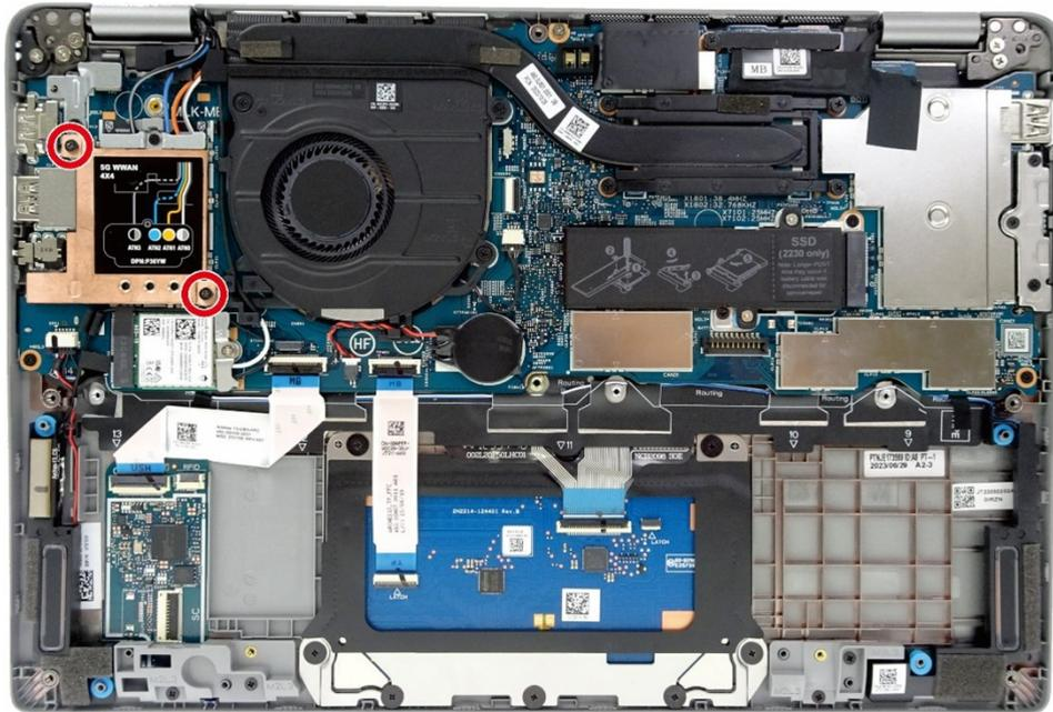
**Figure 33. Metal shielding for the WWAN board**
