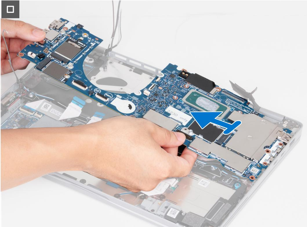
**Figure 47. Removing the system board**
