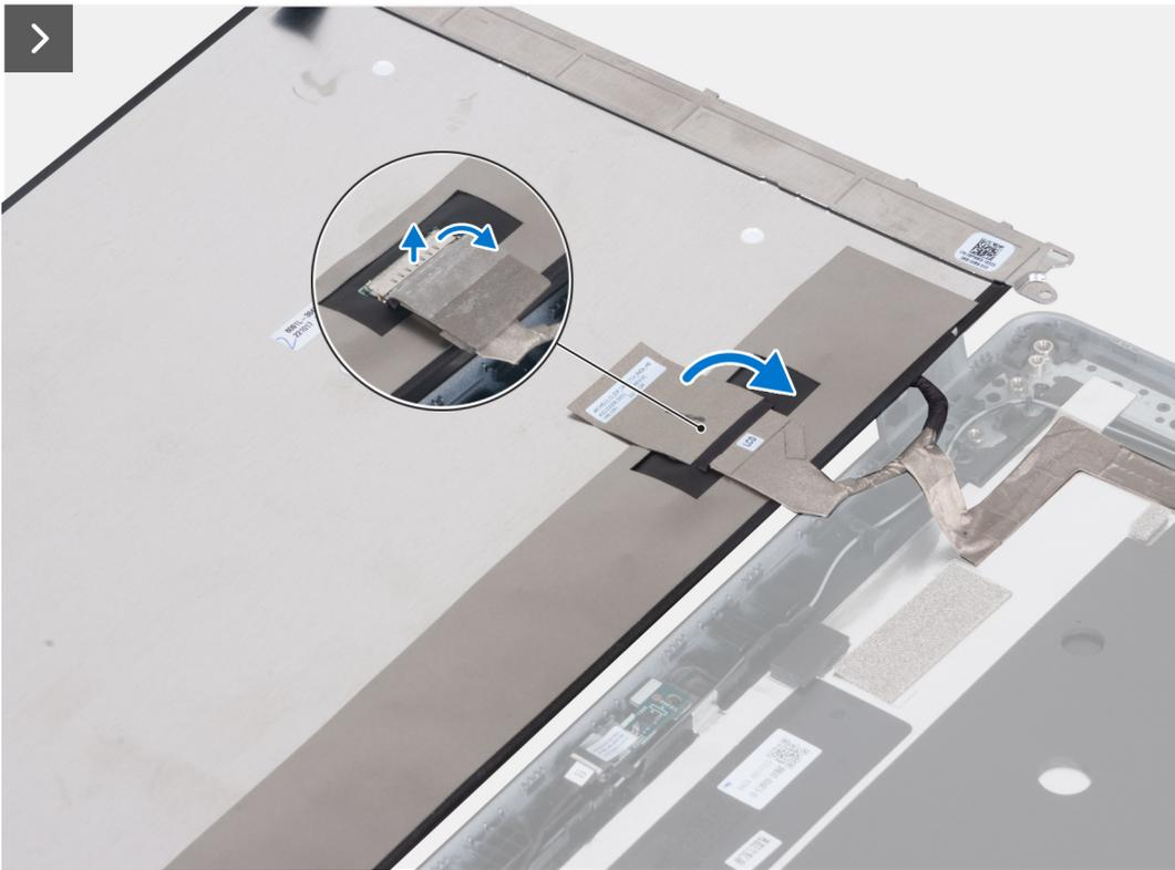
**Figure 75. Removing the display panel (laptop)**
