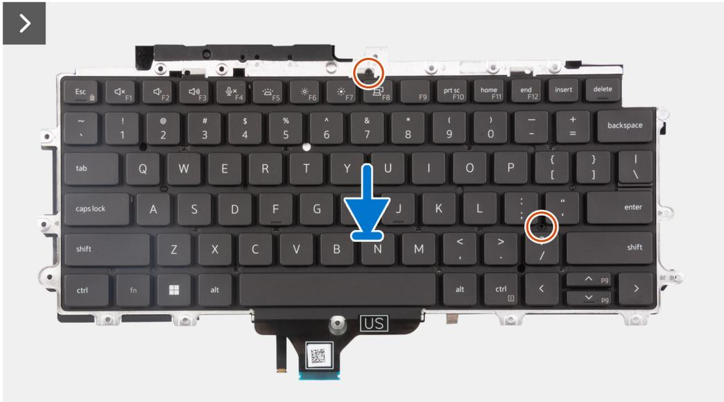
**Figure 61. Installing the keyboard assembly**
