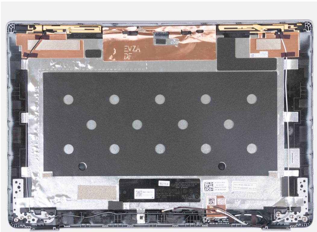
**Figure 84. Removing the display back cover (laptop)**
