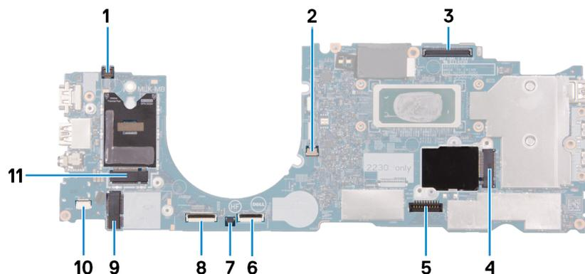
**Figure 44. System-board connectors**
