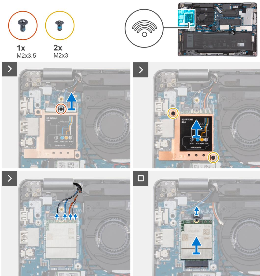
**Figure 30. Removing the WWAN 5G card**
