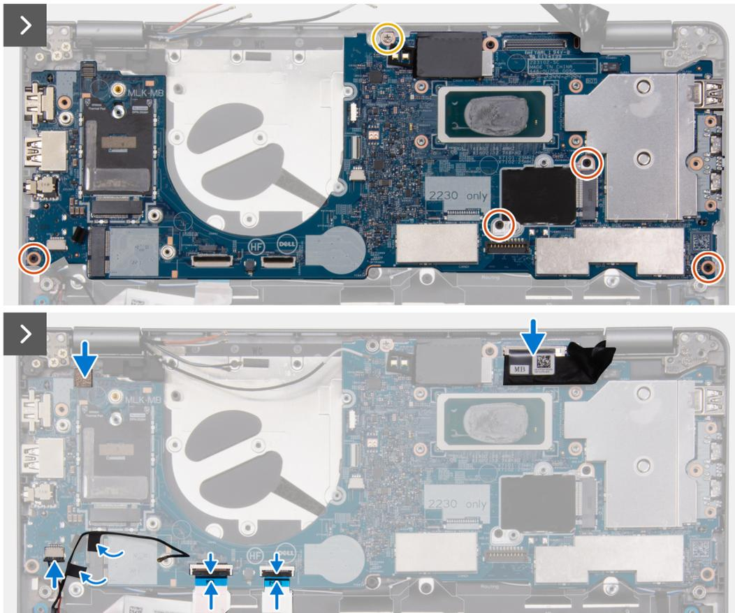
Figure 50. Installing the system board
