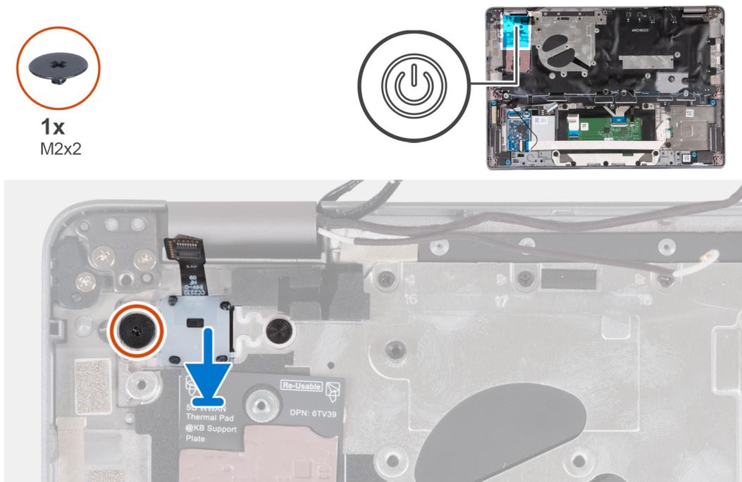
**Figure 58. Installing the power button with fingerprint reader**
