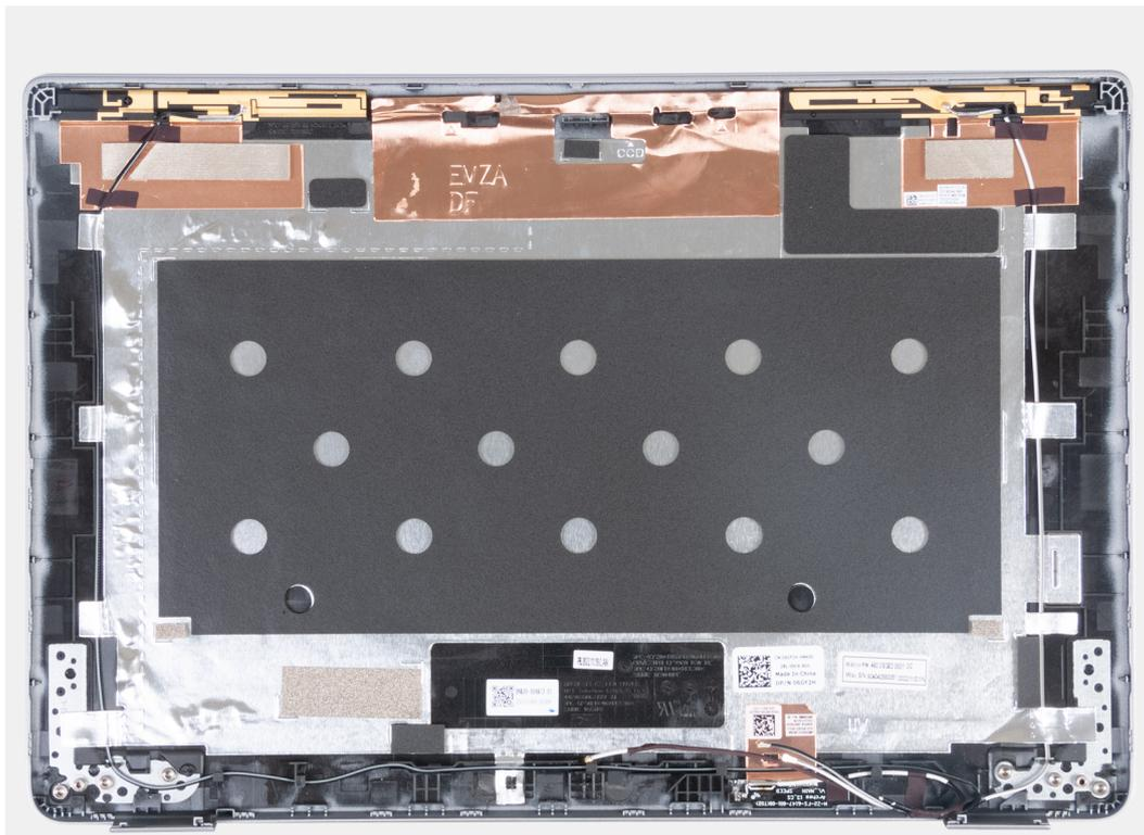
**Figure 85. Installing the display back cover (laptop)**
