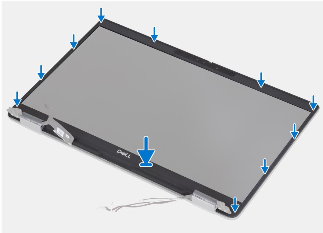
**Figure 69. Installing the display bezel (laptop)**
