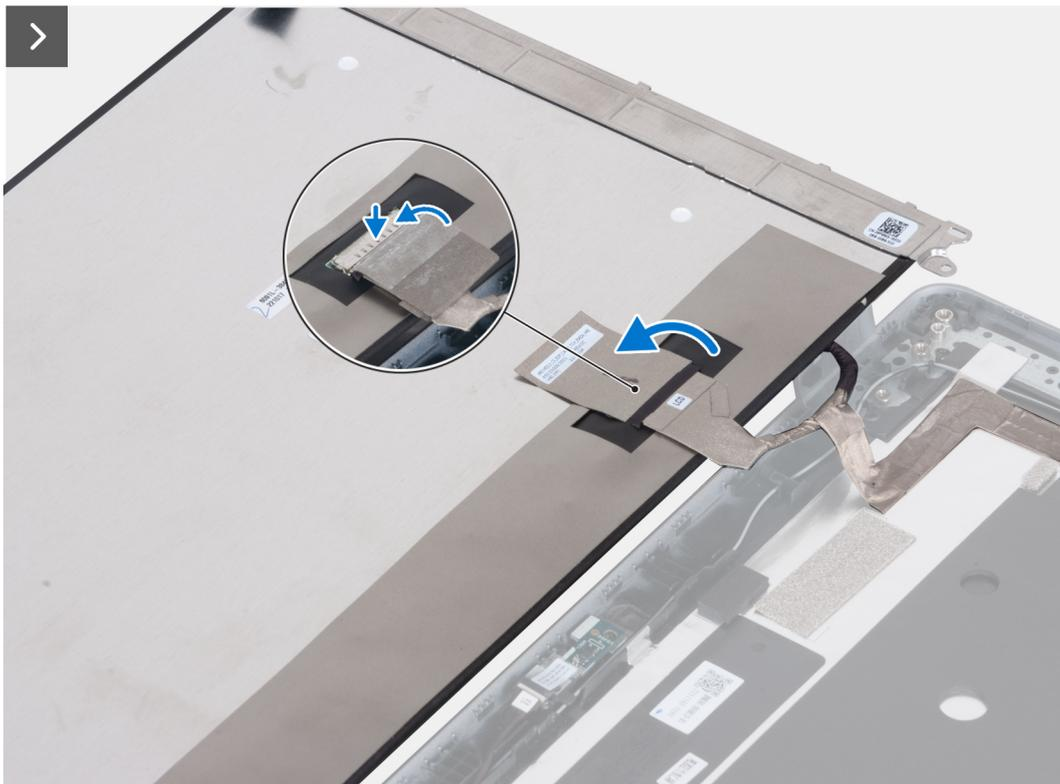
Figure 77. Installing the display panel (laptop)
