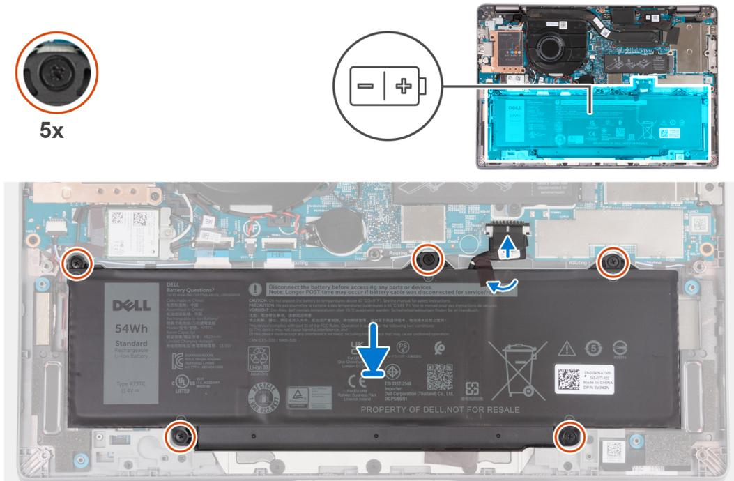
Figure 37. Installing the battery
