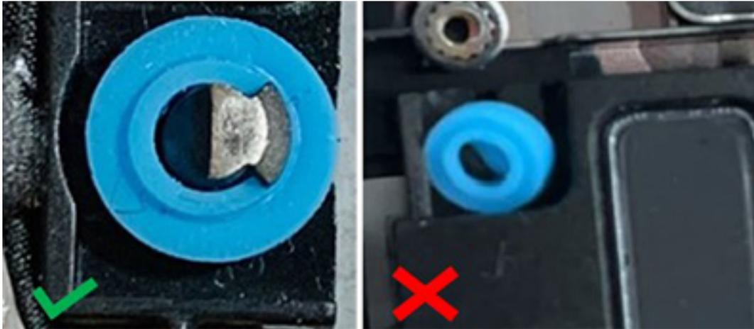
**Figure 54. Rubber grommets of speaker**
