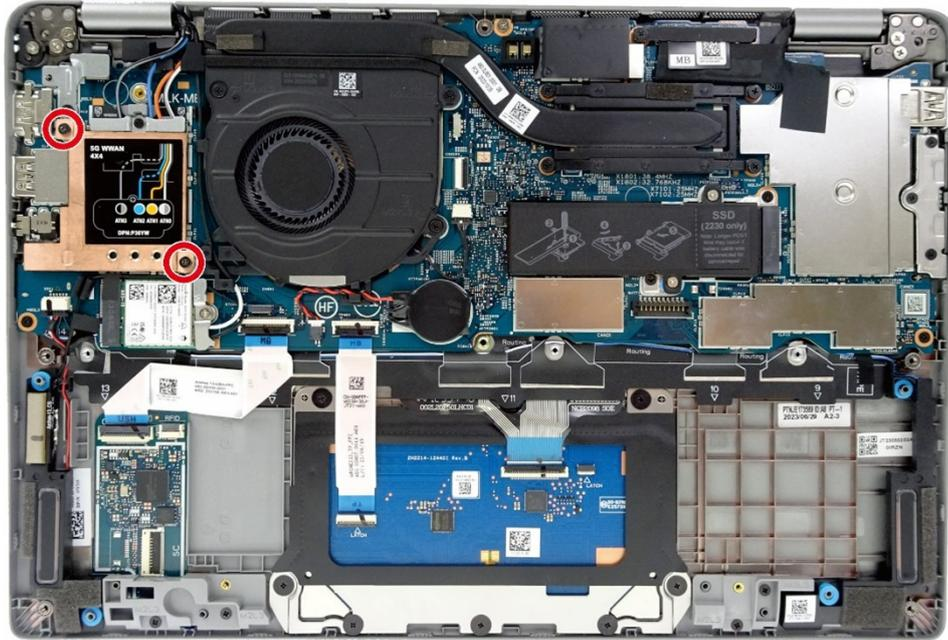
**Figure 31. Metal shielding for the WWAN board**
