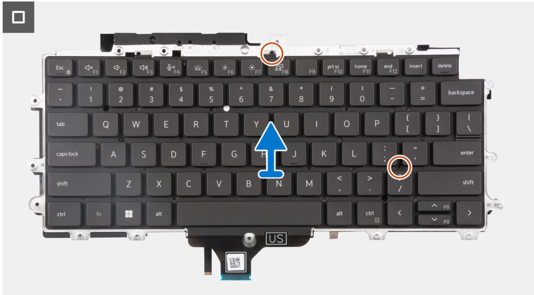
Figure 60. Removing the keyboard assembly
