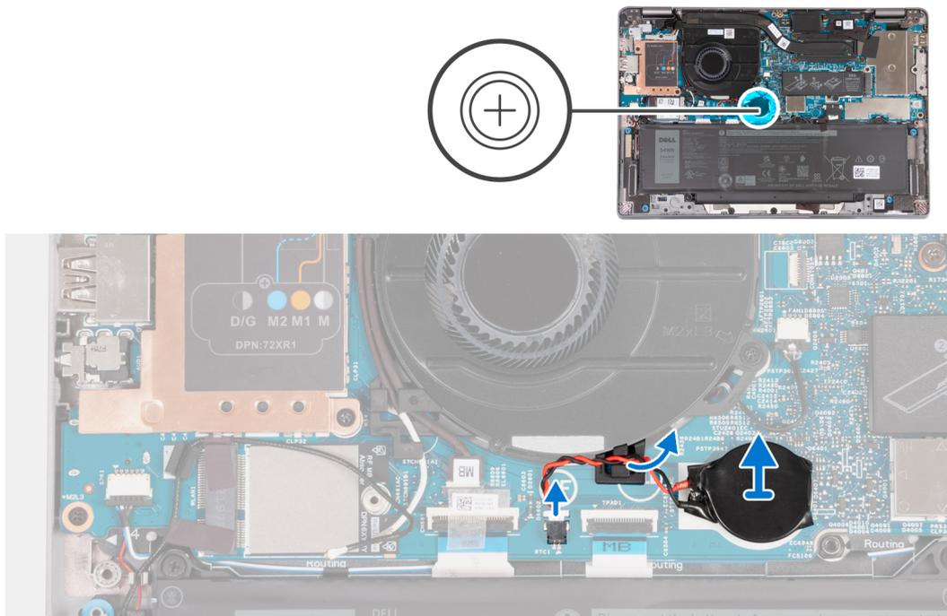
**Figure 40. Removing the coin-cell battery**
