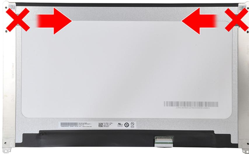
**Figure 73. Stretch Release tape**
