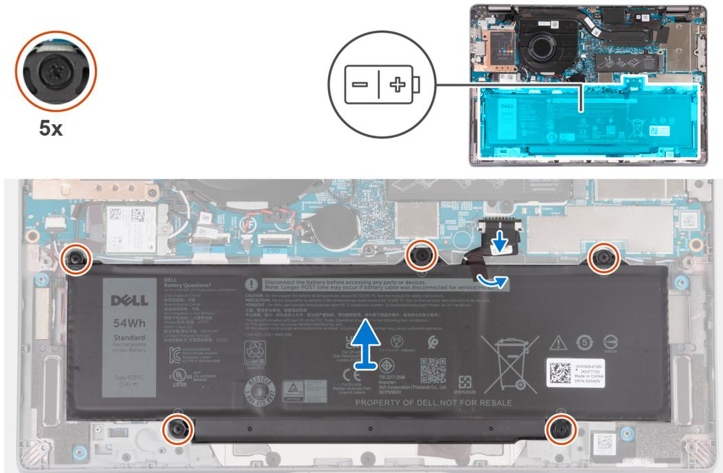
**Figure 36. Removing the battery**
