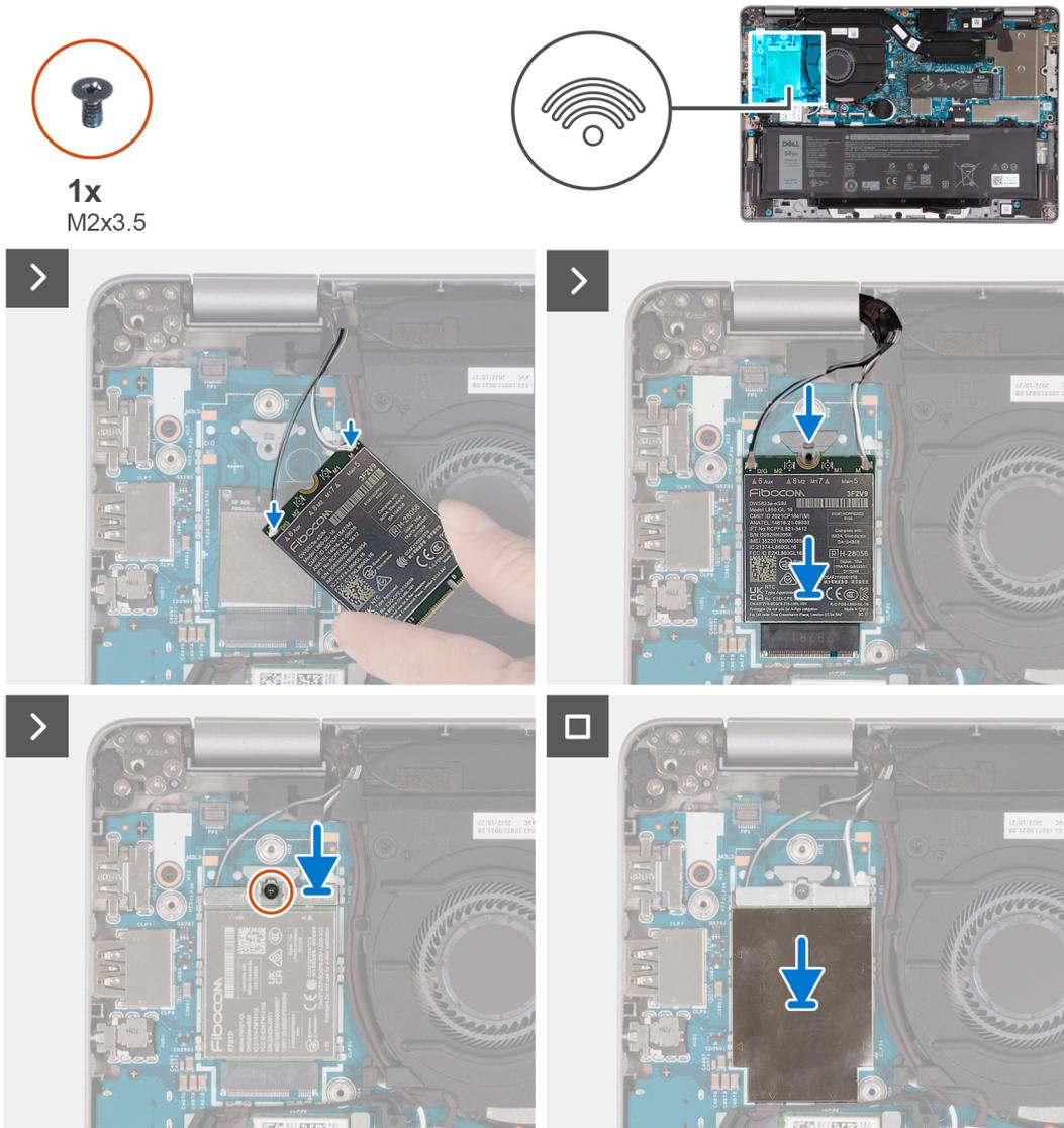
**Figure 29. Install the WWAN 4G card**
