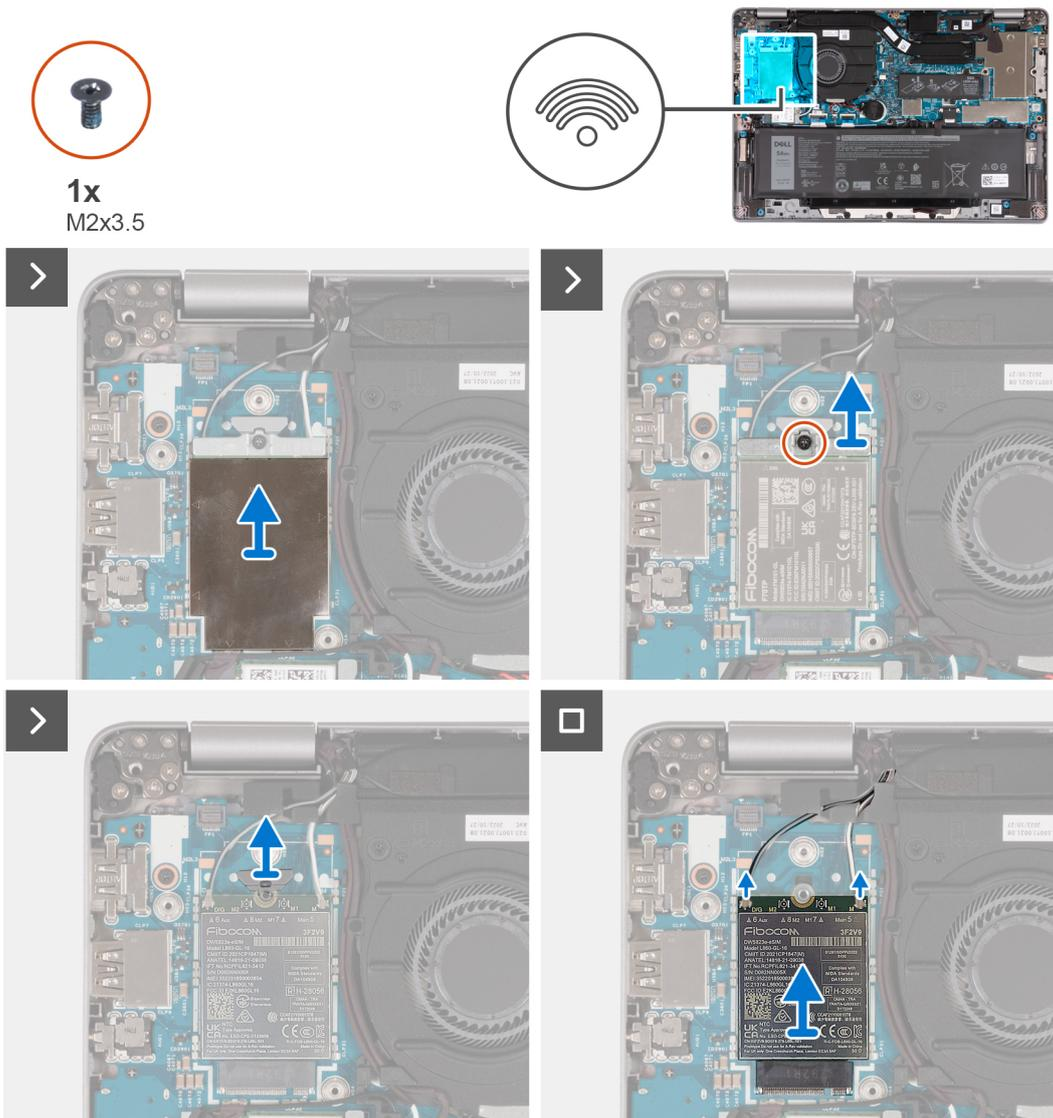
**Figure 28. Remove the WWAN 4G card**
