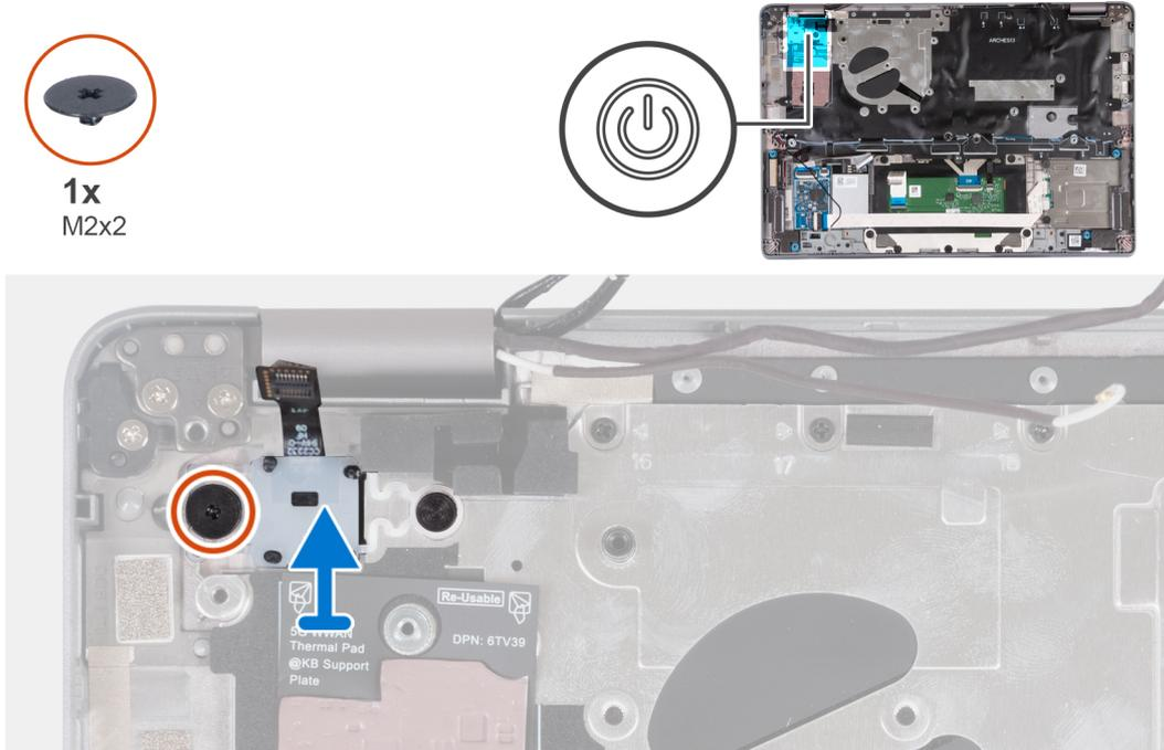
Figure 57. Removing the power button with fingerprint reader
