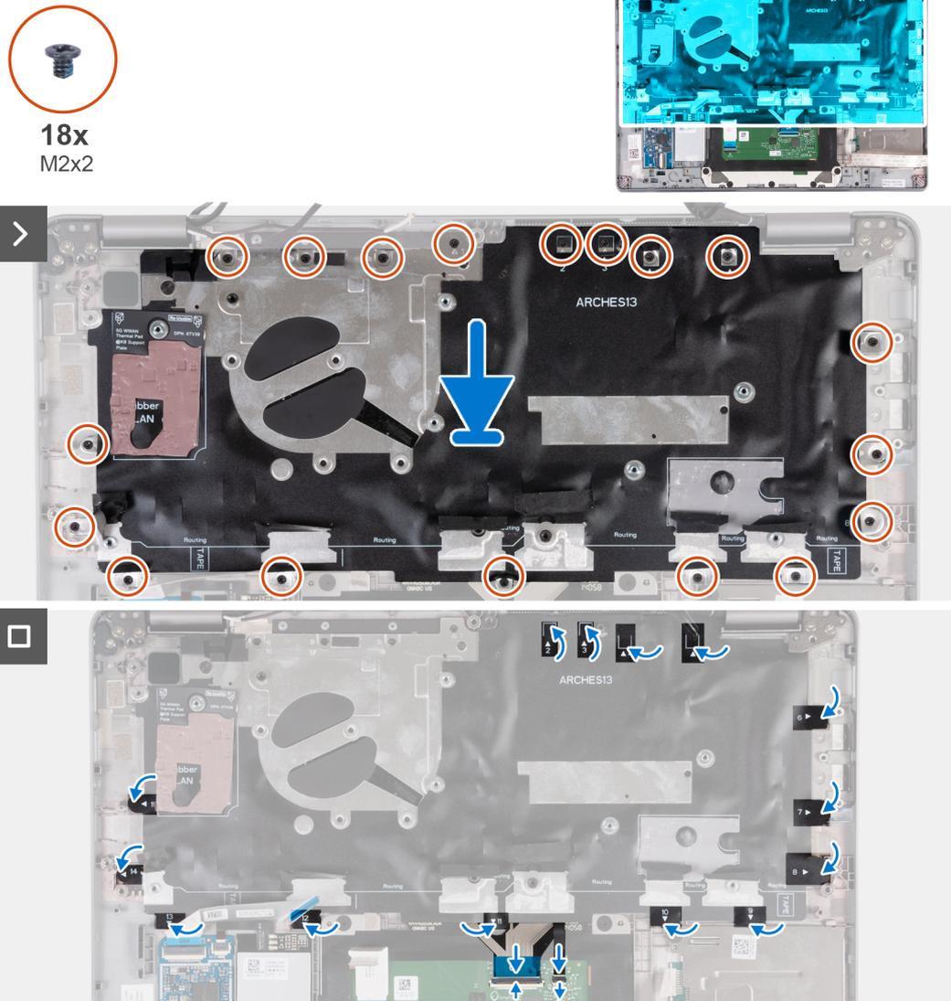
**Figure 62. Installing the keyboard assembly**
