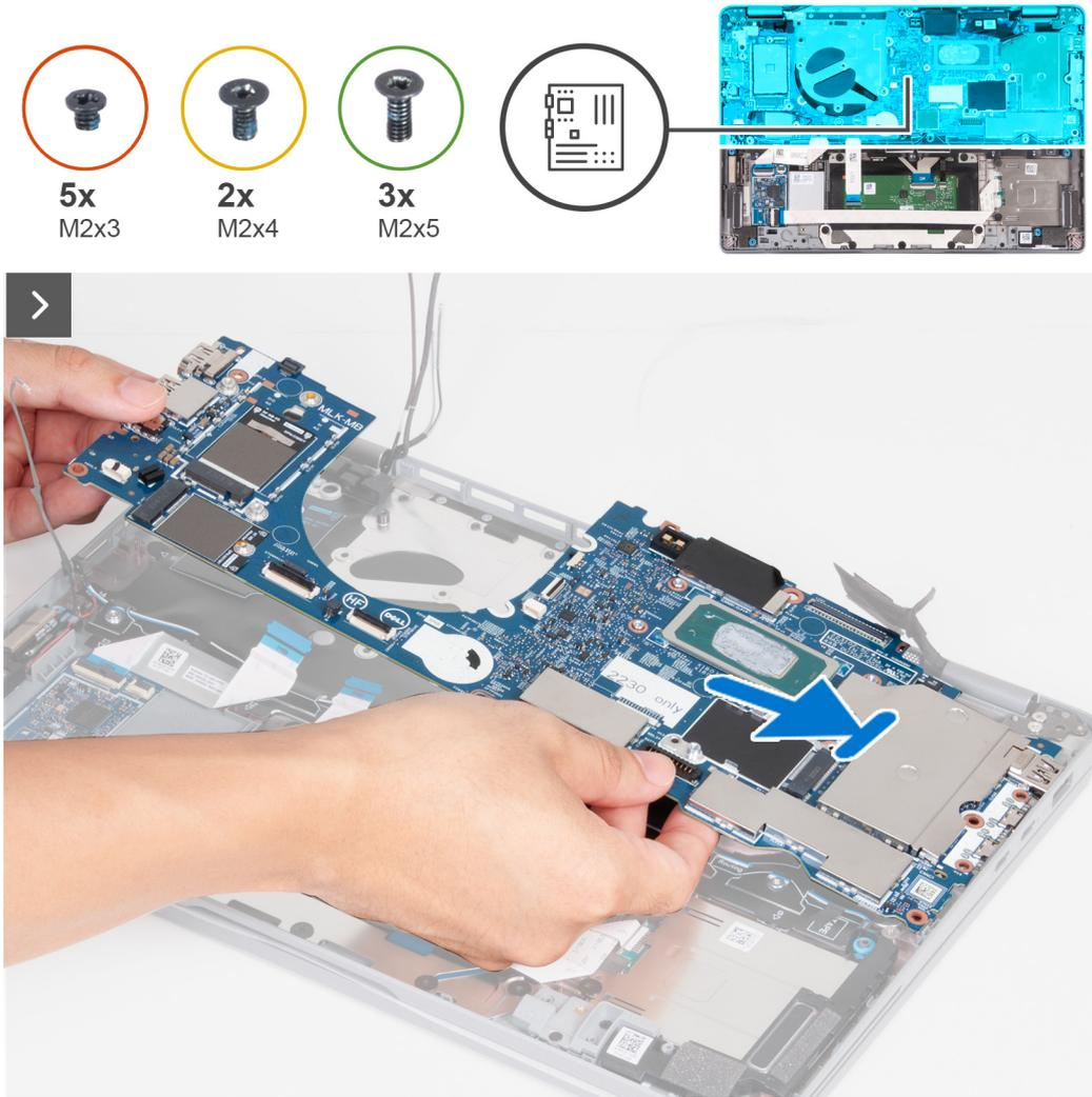
Figure 49. Installing the system board
