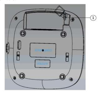
1 Position of the hasps for the locks on the back of the 9117AXI models
