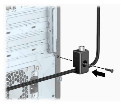
**9.** Insert the plug end of the security cable into the lock **(1)**, and push the button in **(2)** to engage the lock. Use the key provided to disengage the lock.
